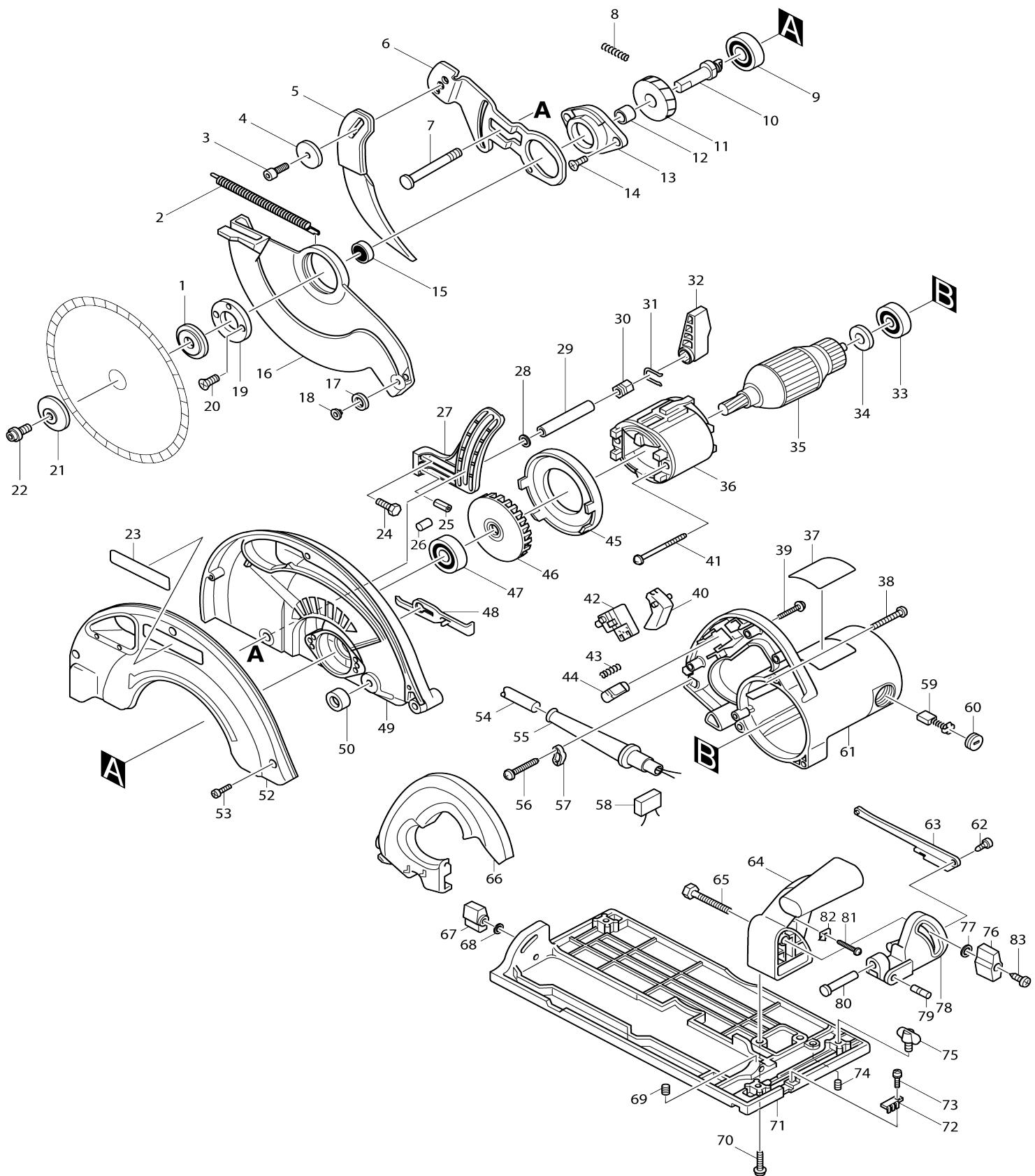
Model No.5903R SCIE CIRCULAIRE 2000W D=235mm
